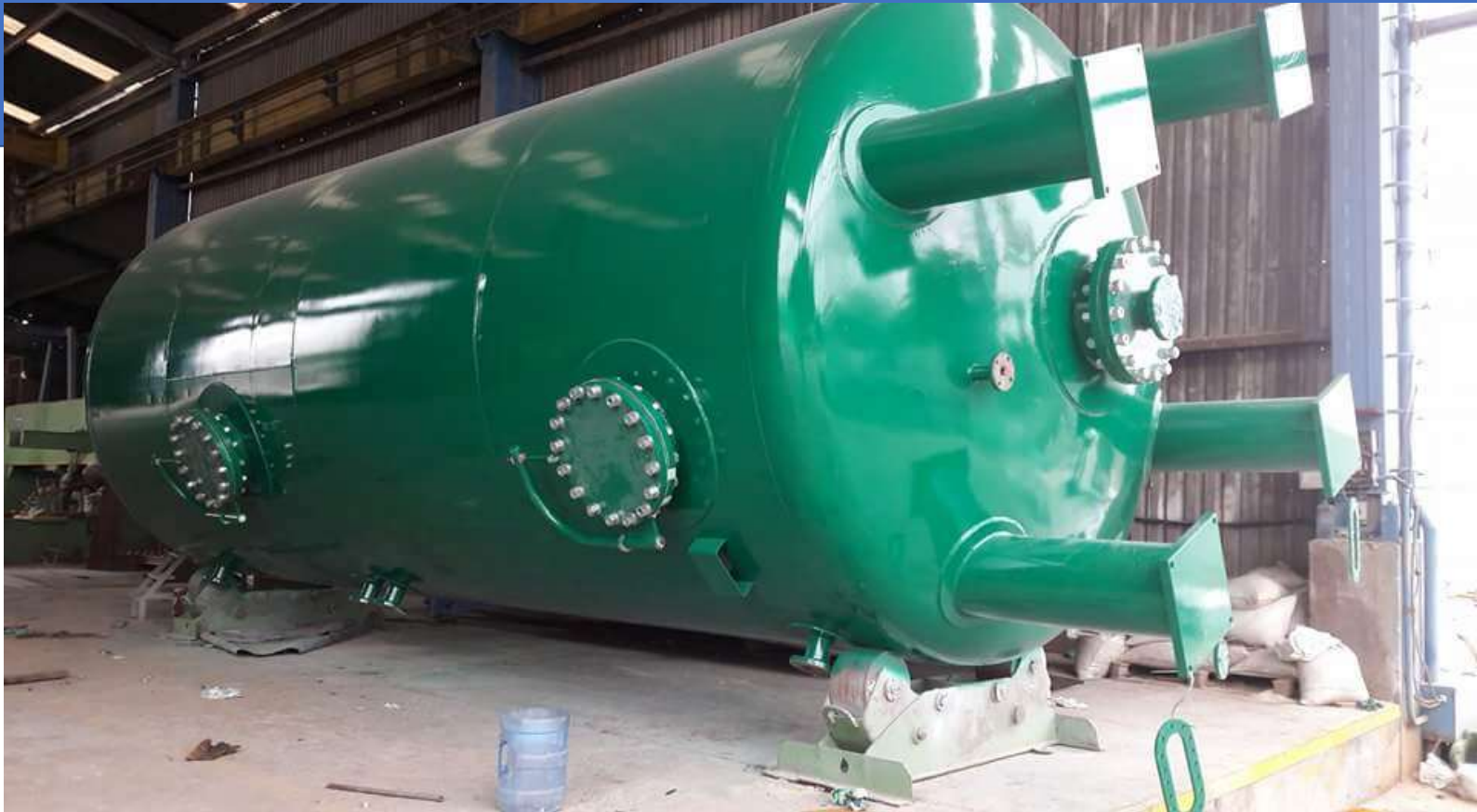
Pressure vessel in carbon steel
