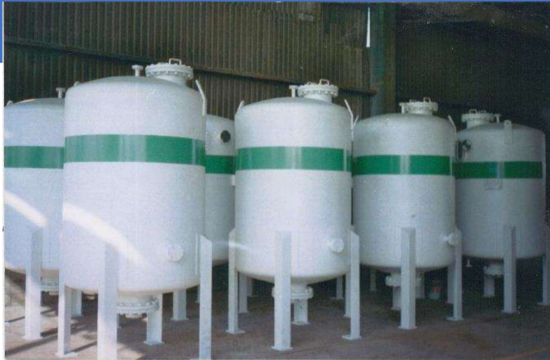
Sand filters in Carbon steel
