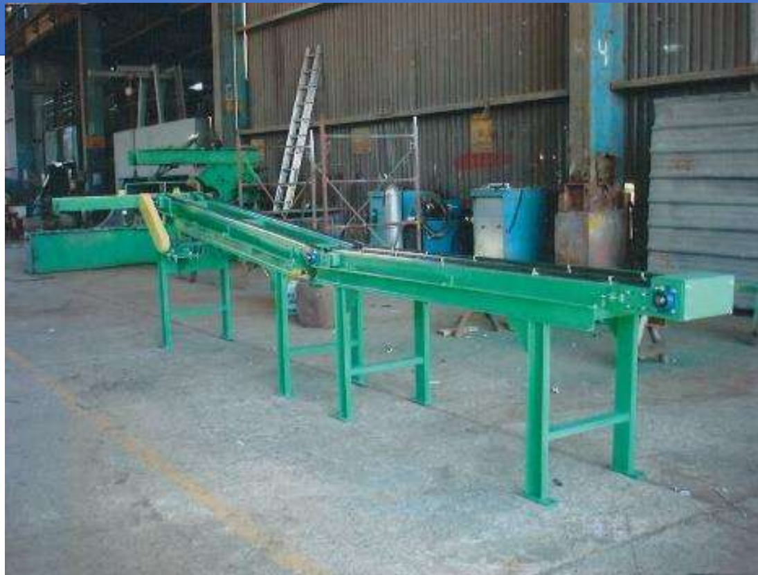
Lead Ingot Conveyor
